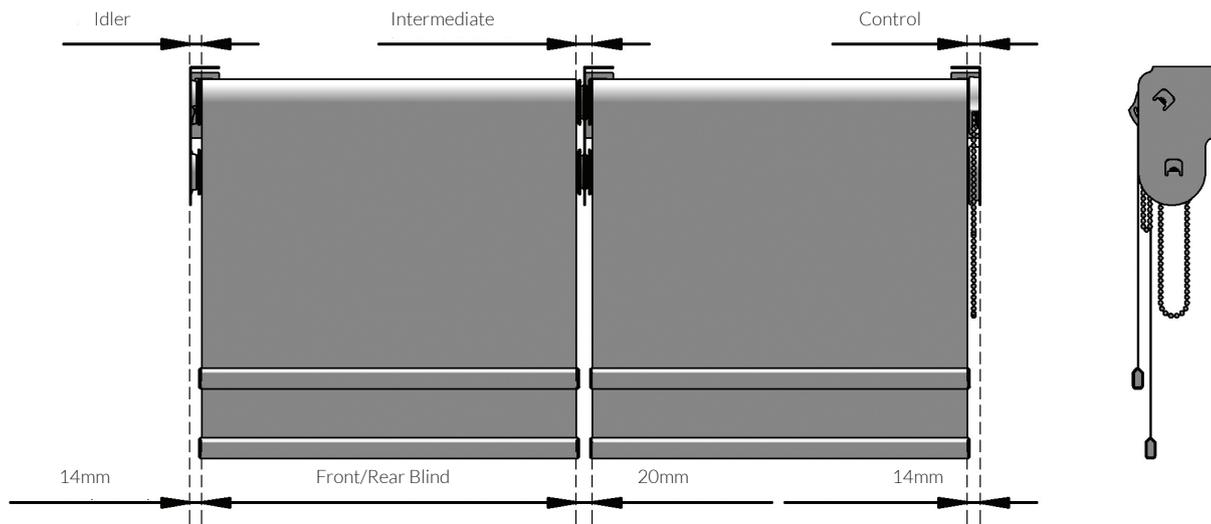
Note: Square Combo brackets are symmetrical. Light gaps on both sides are 14mm as illustrated above [chain op]
